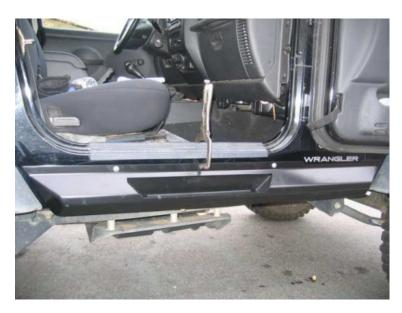
3. With the rocker in place, transfer all holes along the body to be drilled.
