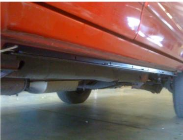
2. With the rail snugly in place. Install the rocker and align along the body.
