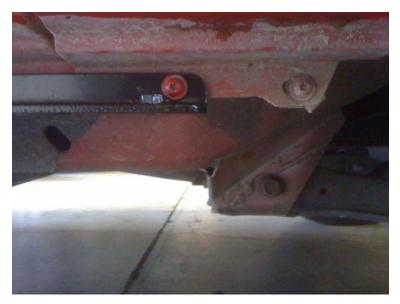
1. Install lower mount rail to the body of the Cherokee as shown.
